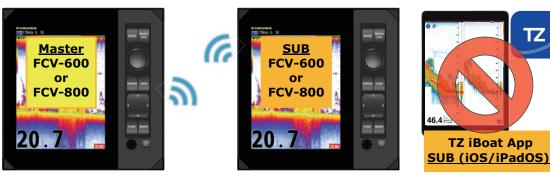
• When the iPhone/iPad is connected to the FCV unit and the TZ iBoat application is used, additional sub-monitor of the FCV cannot be connected.
