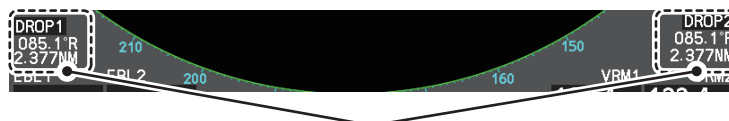
Drop mark boxes show the mark number, bearing and range to the mark.
