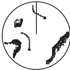
True target trails - Stationary targets are not smeared.
