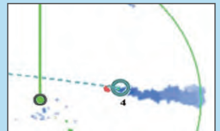
Approaching vessel with target vector and echo trail
